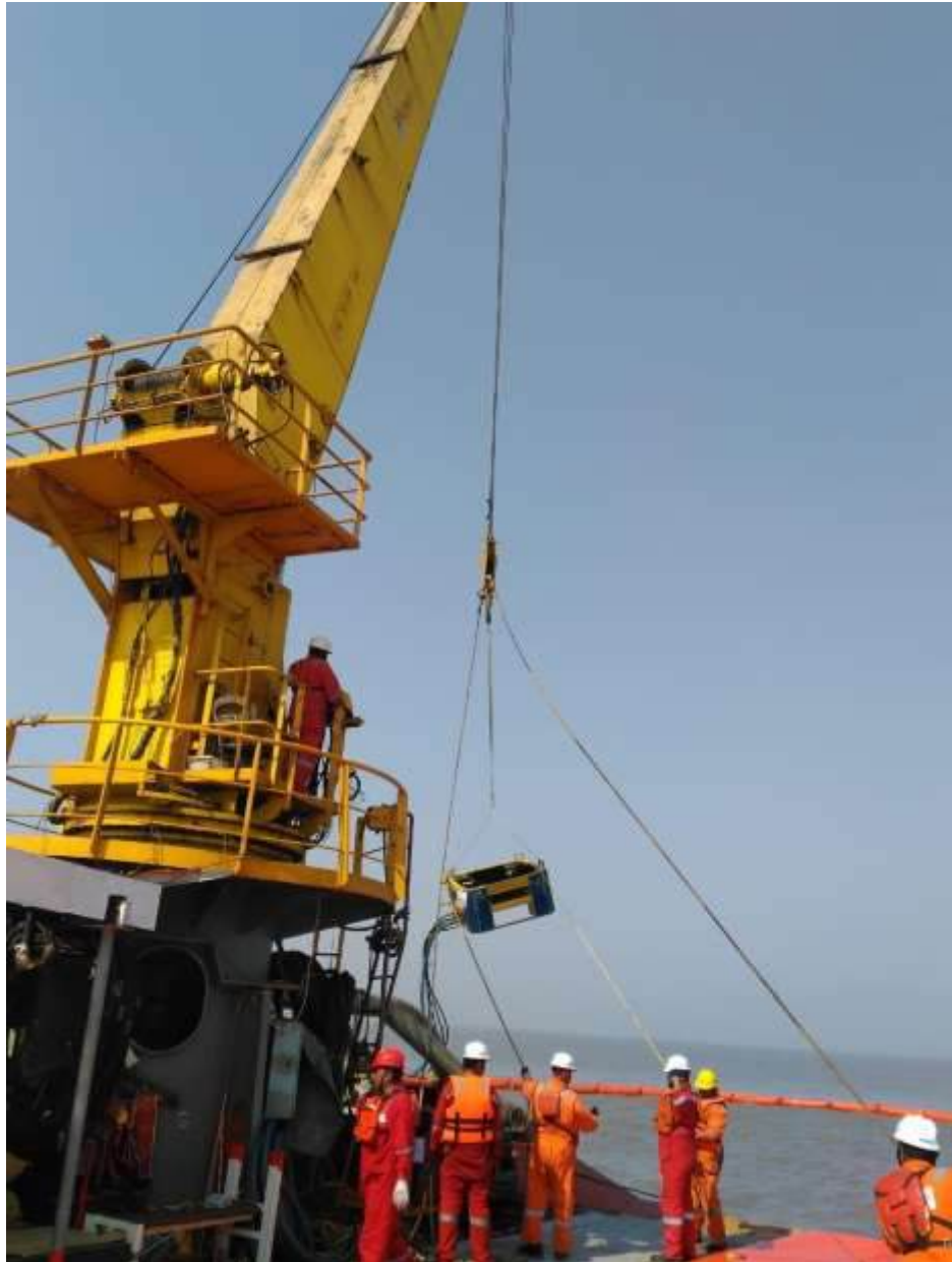
Deployment of Weir Skimmer in Sea
